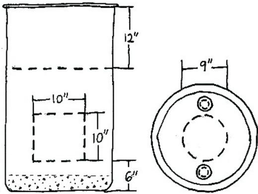
**STEP 1** Using a jigsaw, cut the barrel in two @ 12" from the top of the barrel. Also, cut a 9" diameter round hole in the top and a 10"x10" square hole on the side of the barrel @ 6" above the bottom of the barrel. Following the instructions on the package, Mix the bag of concrete with water and fill the bottom of the barrel with it. Use a trowel to level and smooth out the surface of the concrete.
